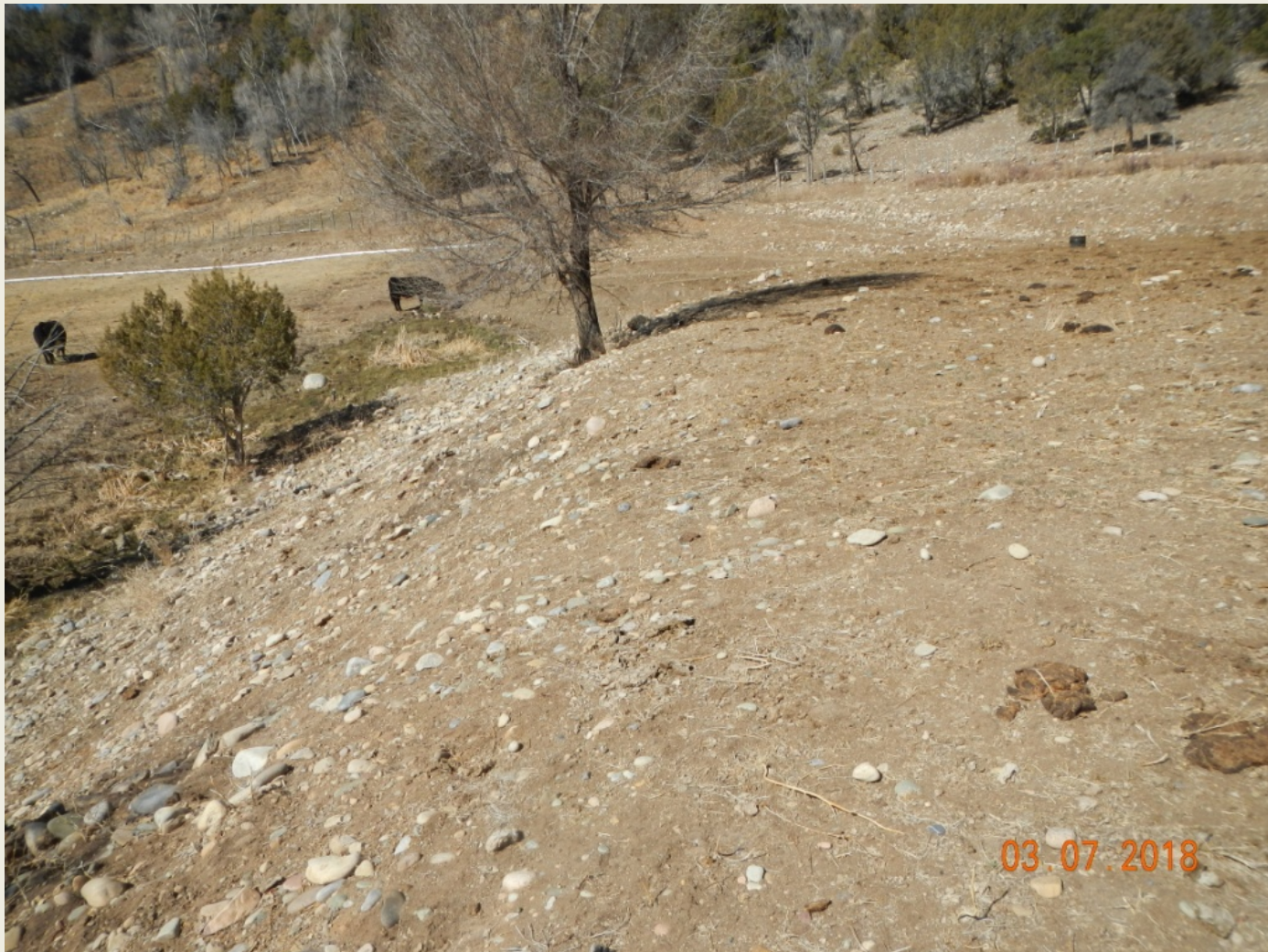
Photo 3. View of the southern portion of the project area from the southeastern corner facing westward. Soils are rocky with little vegetation. Fill is elevated from adjacent contour by approximately 10 to 12 feet.
