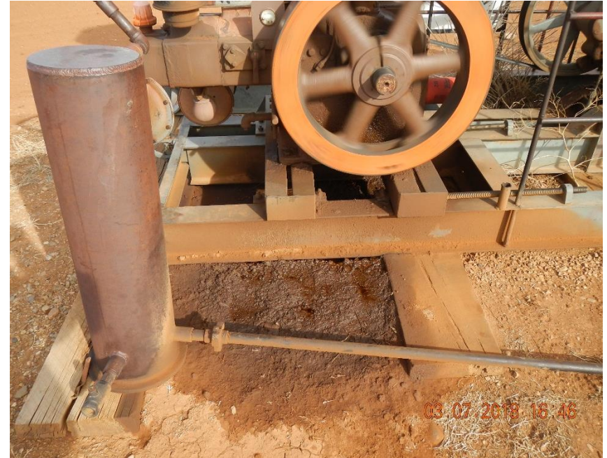
Stained, wet soil underneath prime mover.
