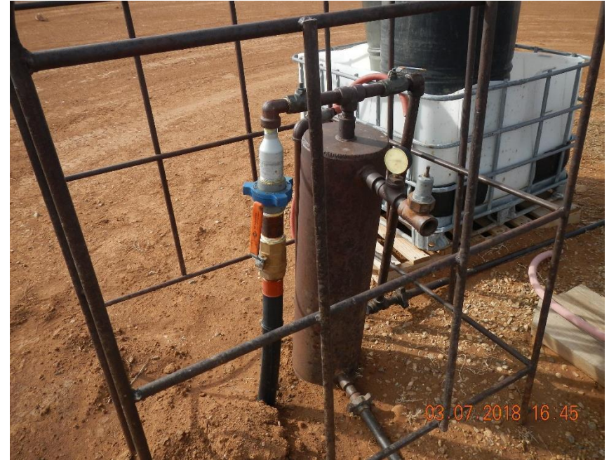
Drop out tank with gas supply line.
