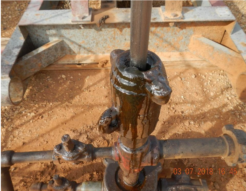
Close up of fluids leaking from well head.
