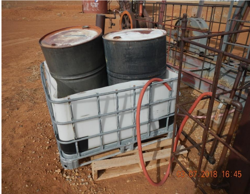
55 gal. drums in secondary containment.
