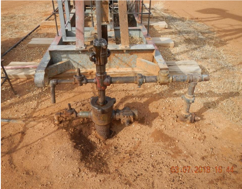
Payne-Schmitt #1 well head and stained soil.
