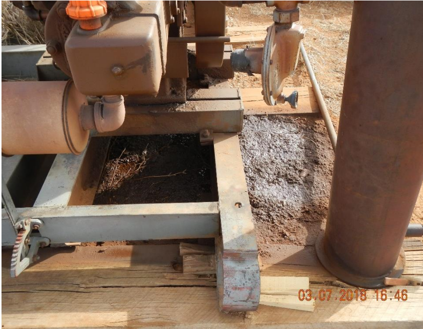
Alternate view of stained soil beneath prime mover.
