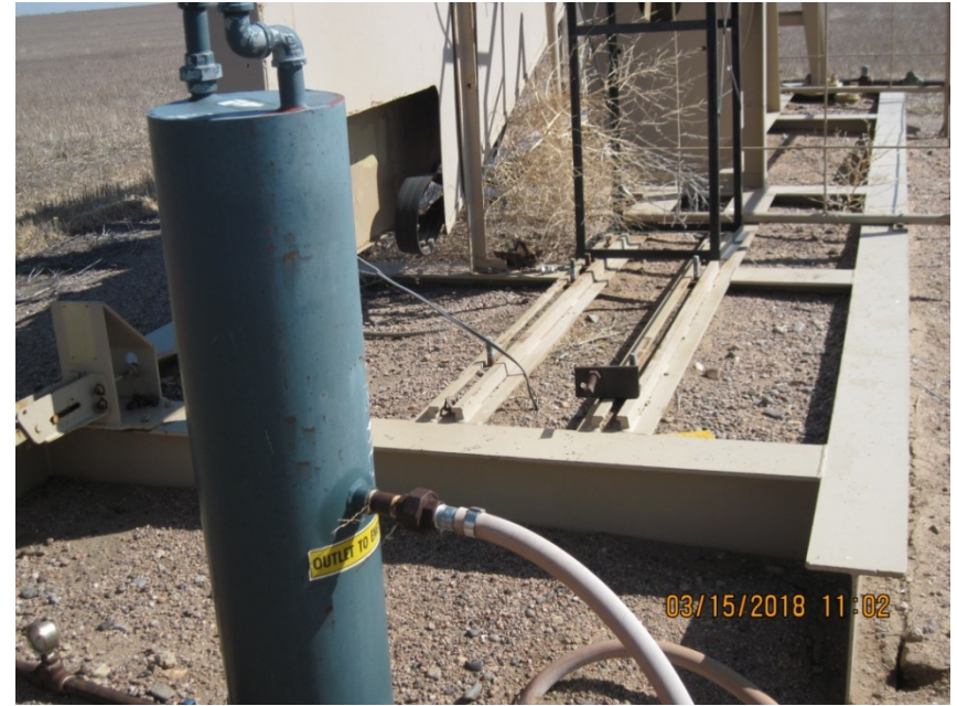
4. Prime mover has been removed
