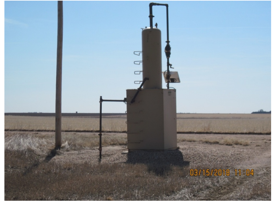
2. Meter shed with vertical gas separator
