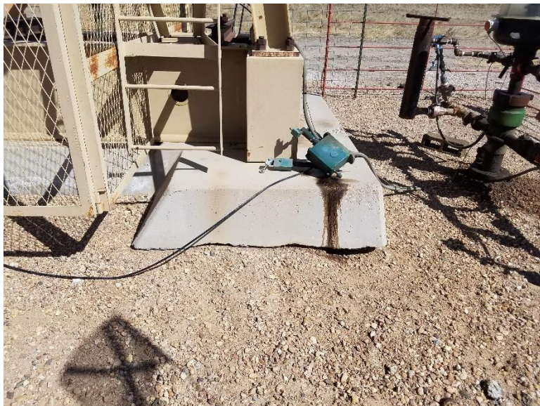
Photo 7. Unused equip. leaking fluid to ground
