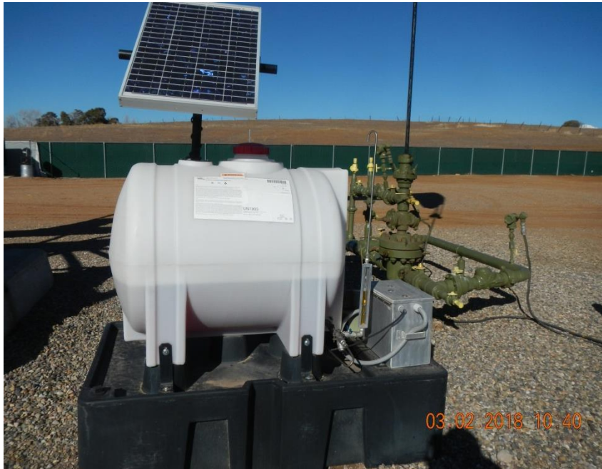
Chemical injection system labeled combo inhibitor without NFPA placard filled out.
