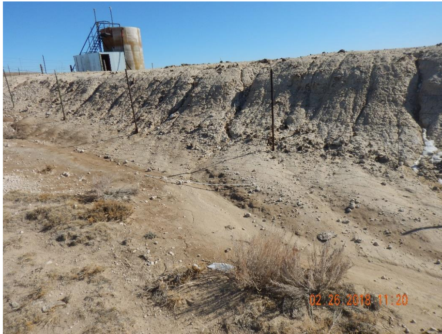
Photo 17: Photo taken from the west end of the pit, facing east. Photo shows stormwater runoff has caused erosion degradation at the pit walls, which has then contributed to degraded to the adjacent areas.
