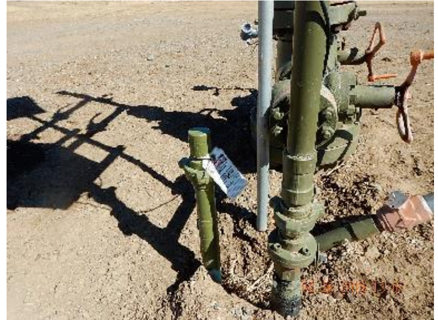
Photo 2: Unused riser at wellhead.
