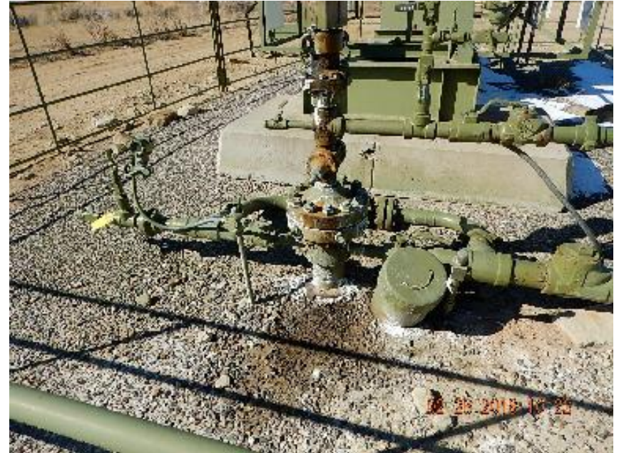
Photo 10: Impacted soil at wellhead current inspection.
