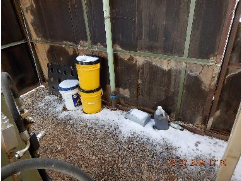
Photo 5: Supplies stored at wellhead compressor with no spill prevention.
