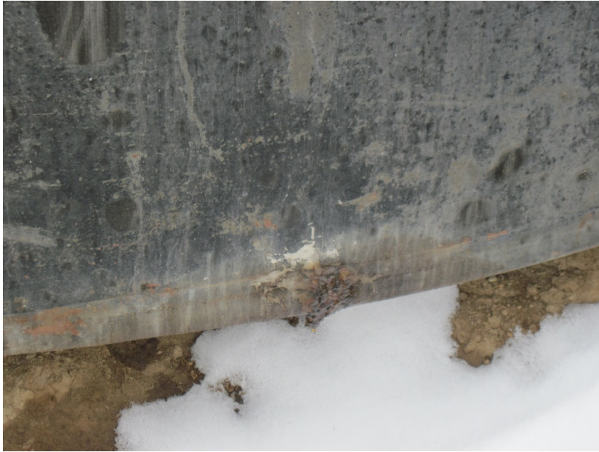
HOLE IN PROD TANK
