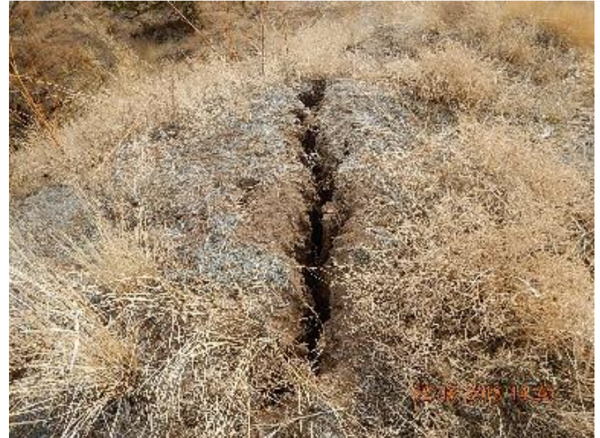
Photo 4: Soil separation at SE corner.
