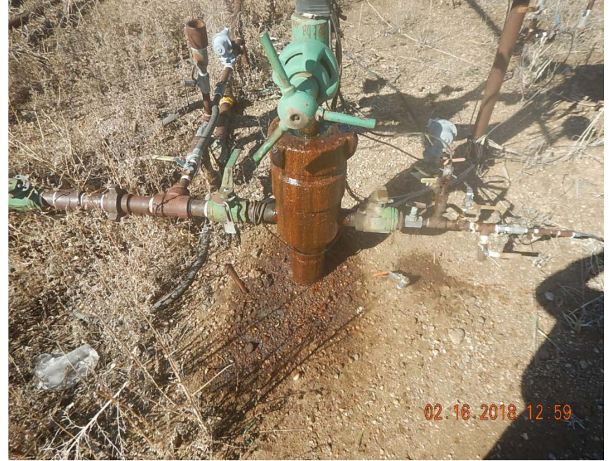
Photo 3: Stained soil at wellhead, leaking at wellhead
