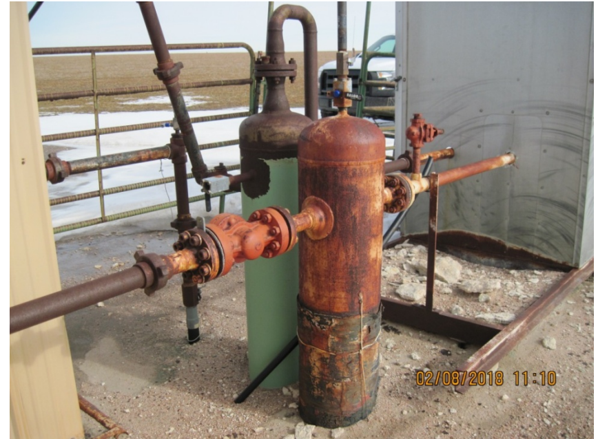
4. Vertical gas separators 50% buried
