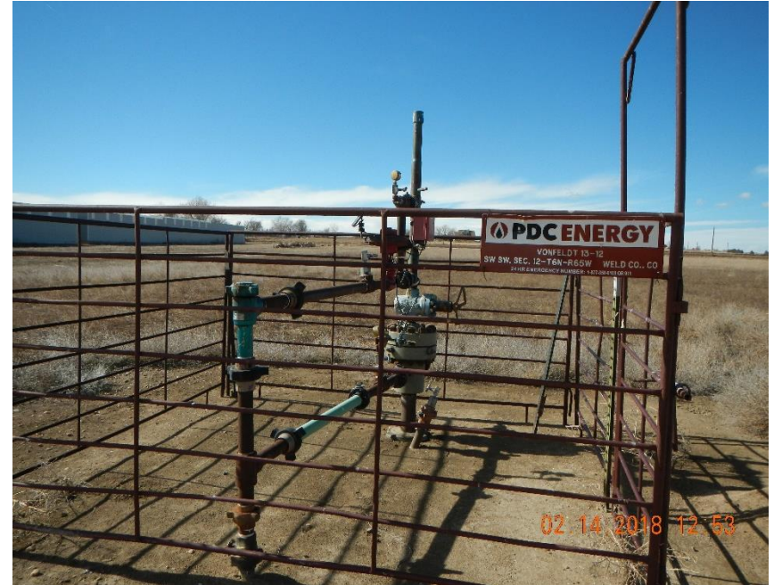
Wellhead and signage
