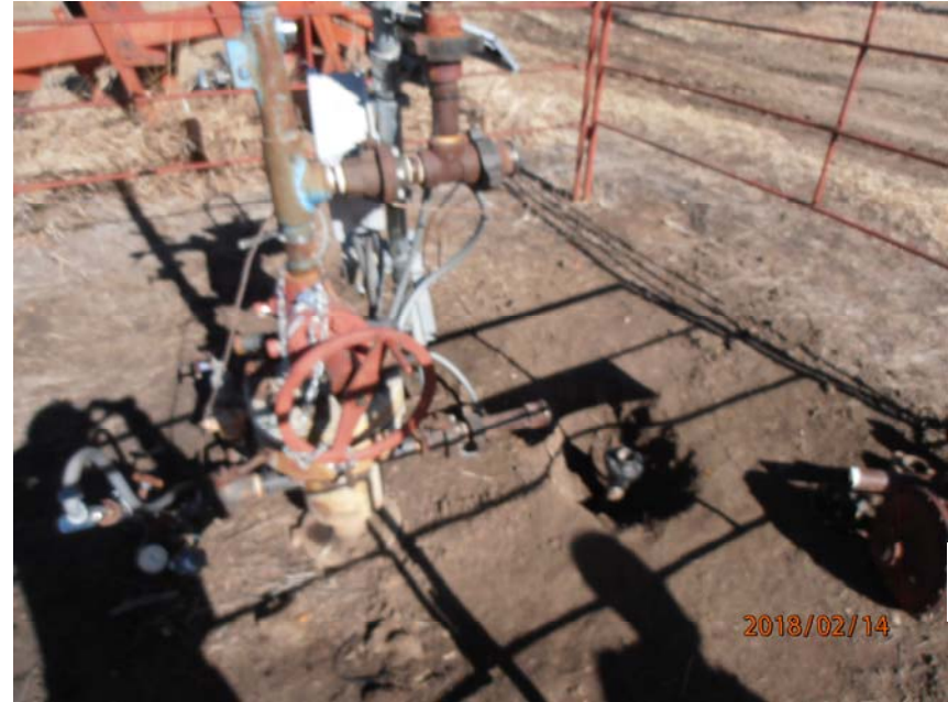
Photo 4 – with riser disconnected from wellhead.
