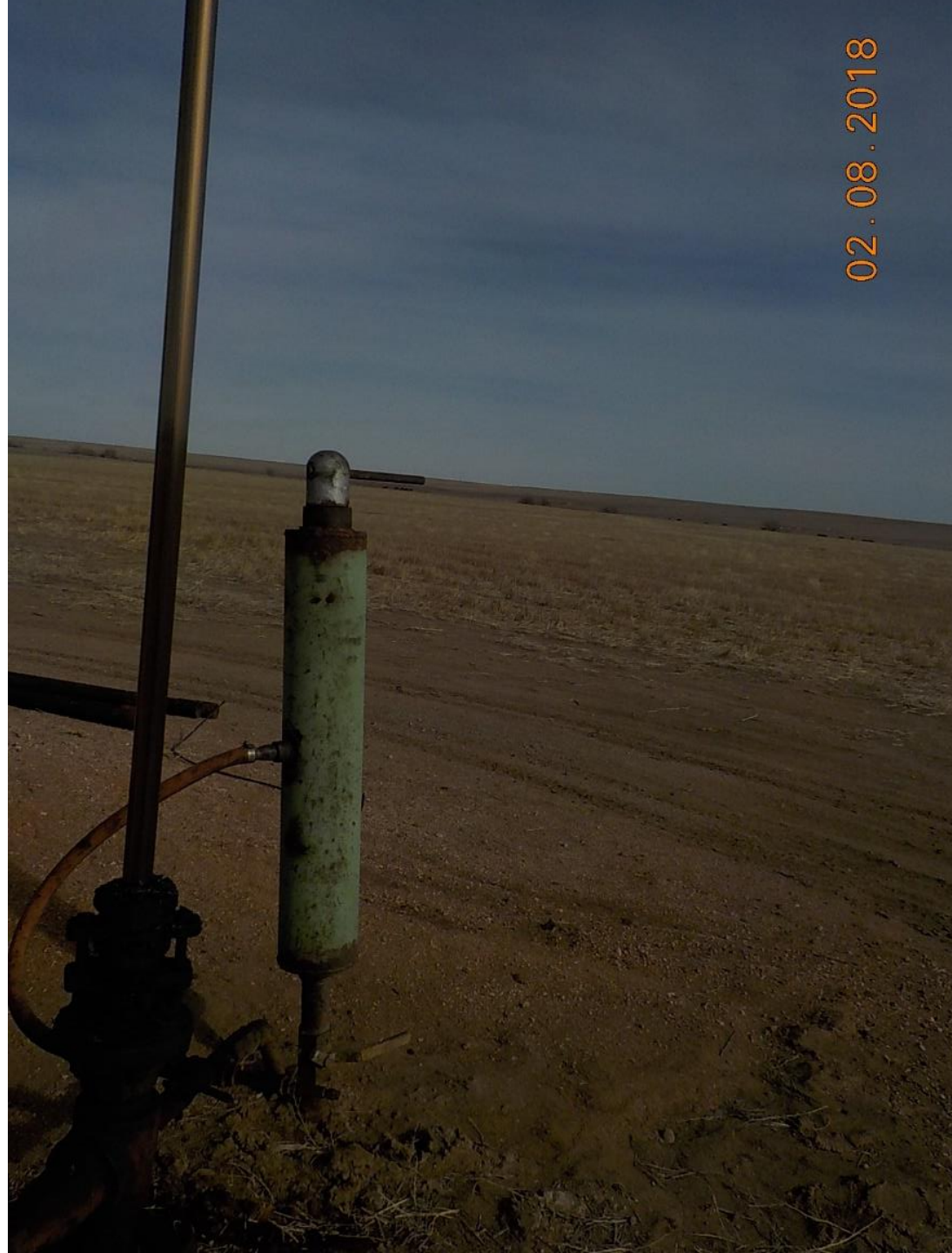
Stained soil at wellhead.
