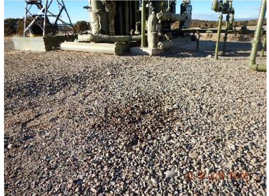
Photo 6: Impacted soil and gravel between compressor and gas meter runs.
