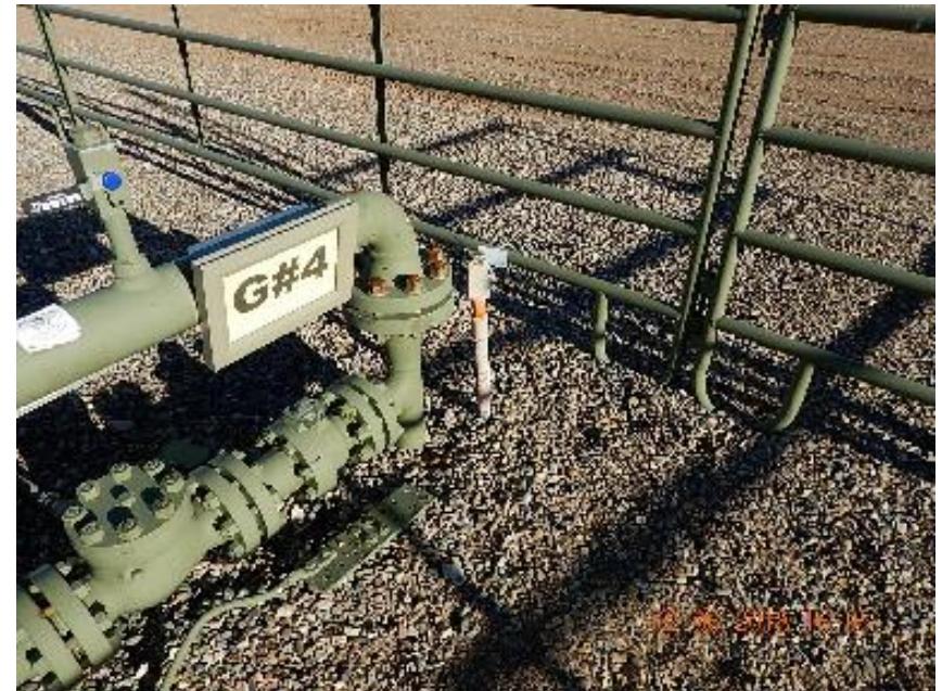
Photo 2: Unused supply gas riser at G#4 wellhead.
