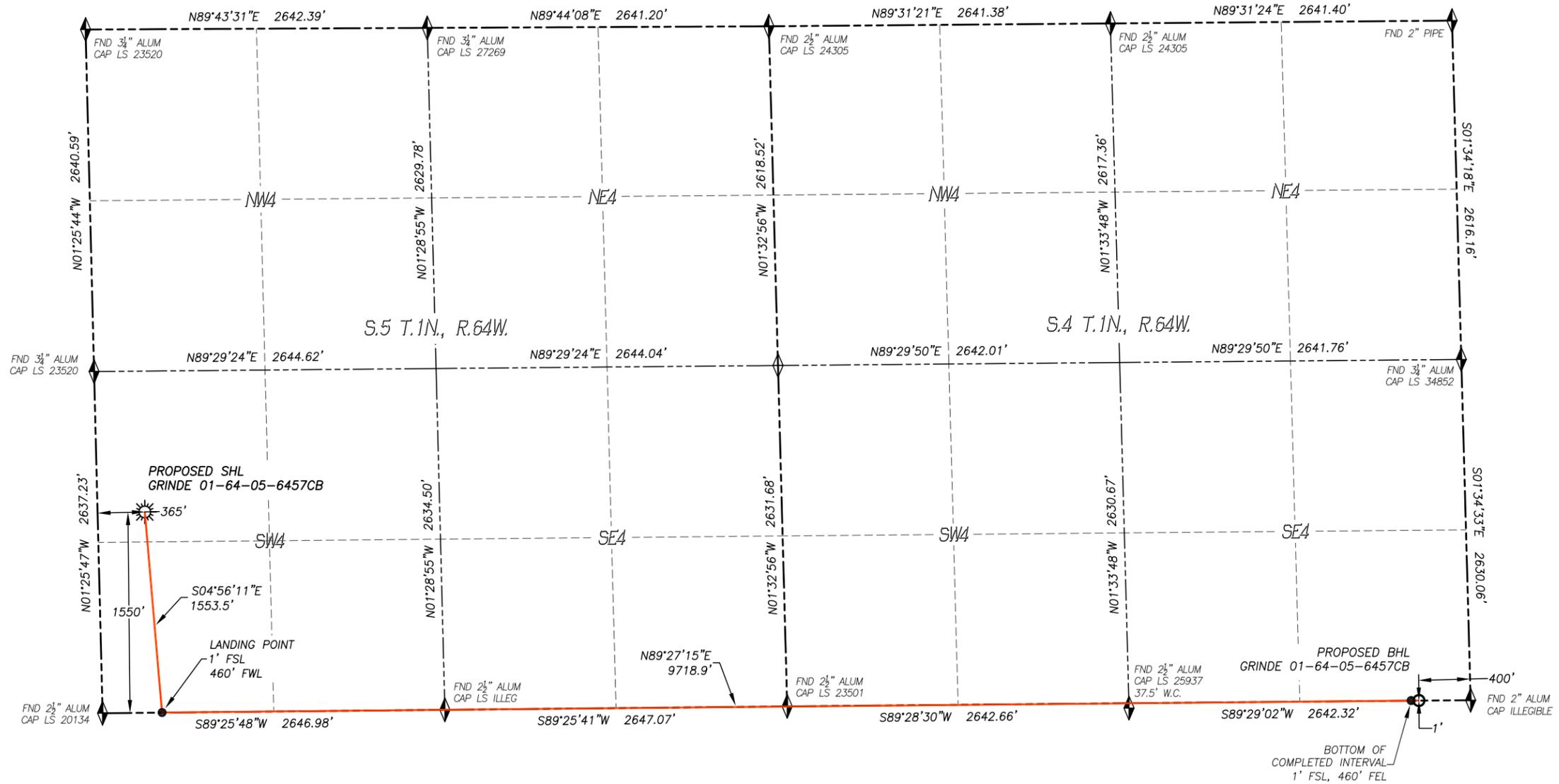
IN ACCORDANCE WITH A REQUEST FROM BILL BARRETT CORP., DALEY LAND SURVEYING, INC. HAS DETERMINED THE SURFACE LOCATION OF THE GRINDE 01-64-05-6457CB WELL TO BE 1550' FSL, 365' FWL, AS MEASURED AT NINETY (90) DEGREES FROM THE SECTION LINES OF SECTION 5, TOWNSHIP 1 NORTH, RANGE 64 WEST AND THE BOTTOM HOLE LOCATION TO BE 1' FSL, 400' FEL, AS MEASURED AT NINETY (90) DEGREES FROM THE SECTION LINES OF SECTION 4, TOWNSHIP 1 NORTH, RANGE 64 WEST, OF THE 6TH PRINCIPAL MERIDIAN, WELD COUNTY, COLORADO.
