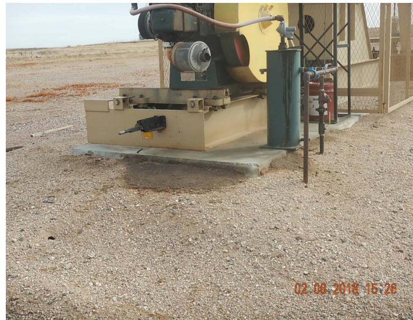
Photo 4: Stained soil at engine
