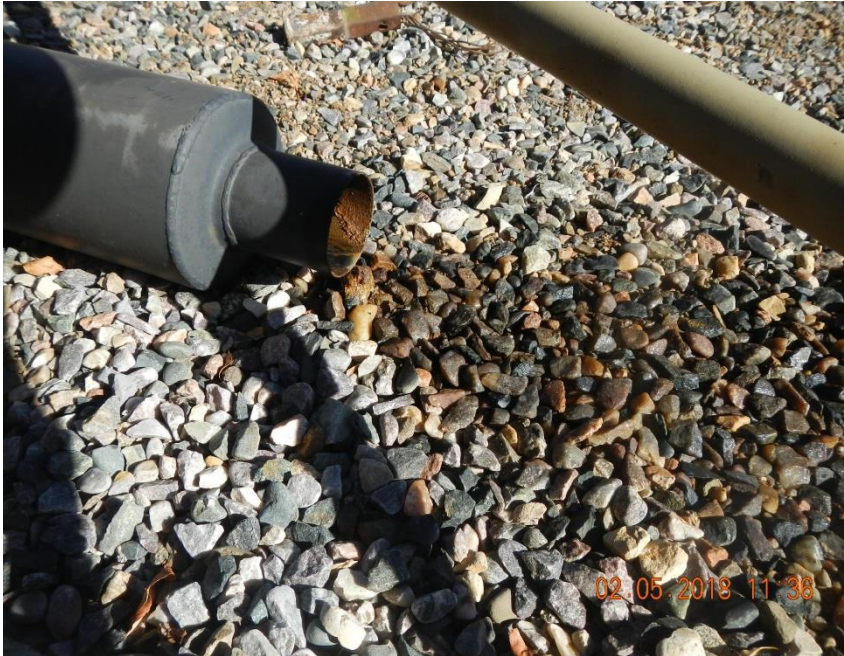
Stained gravel at muffler exhaust.
