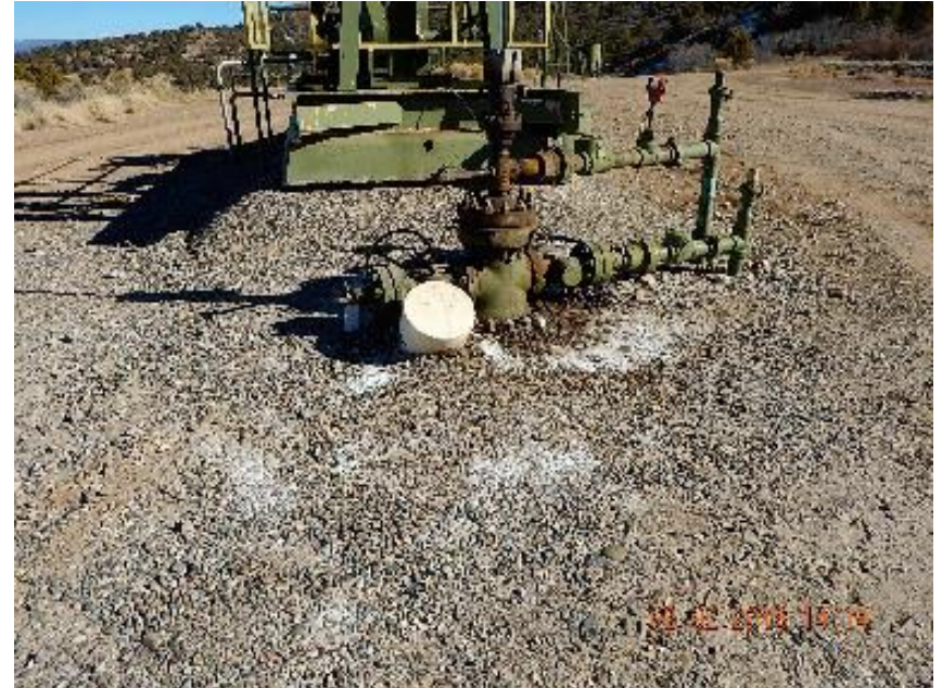
Photo 4: Impacted soil around wellhead.
