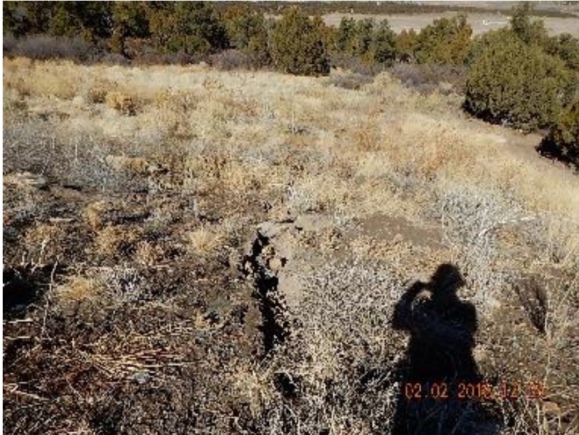
Photo 9: Erosion channel on fill slope.
