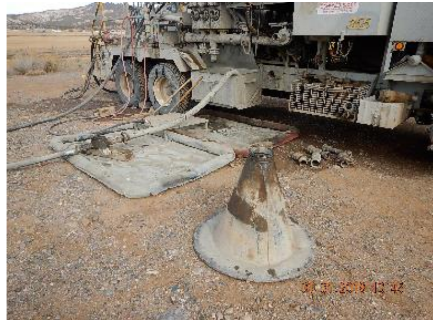
Photo 2: Containment at pump truck.
