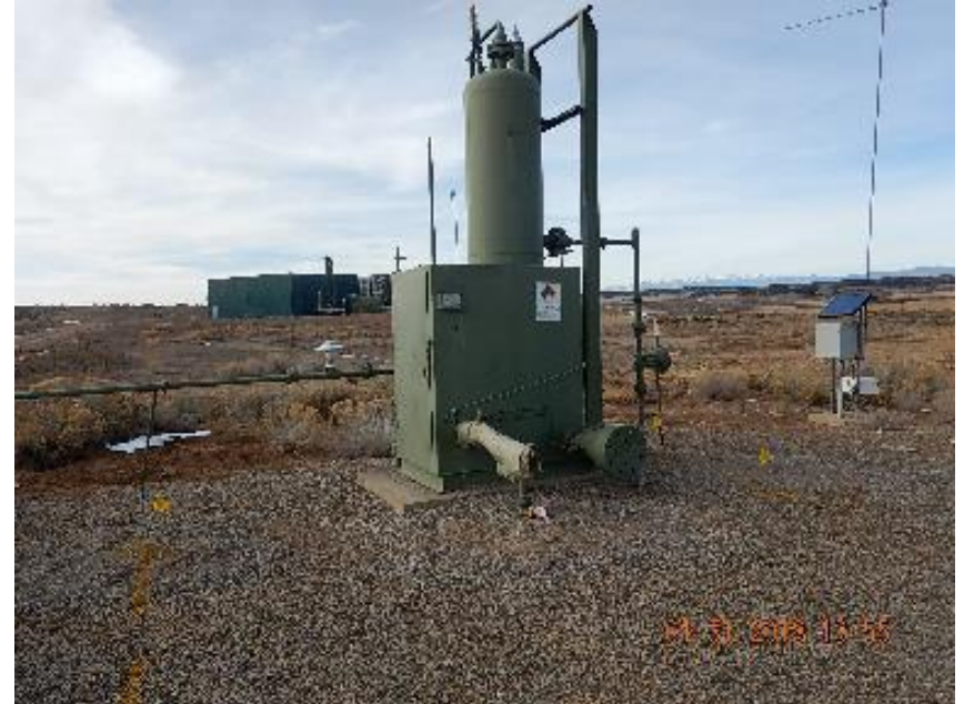
Photo 6: Vertical separator.
