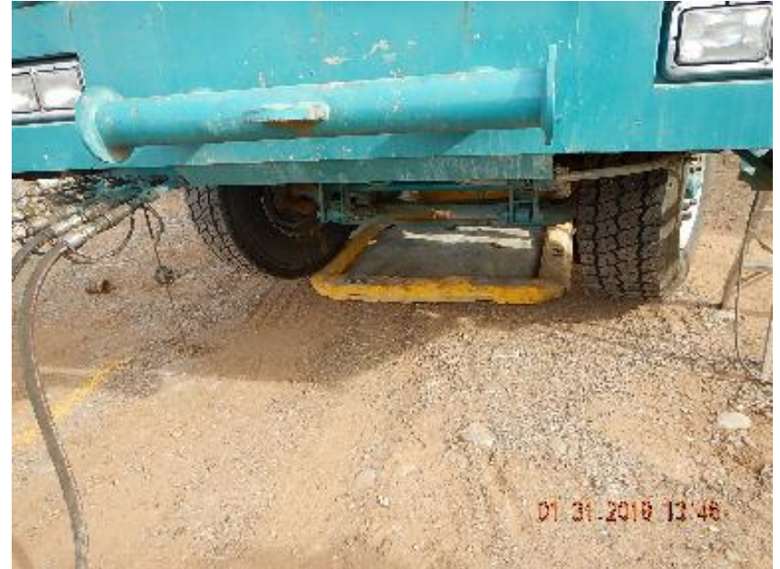
Photo 4: Containment under rig.
