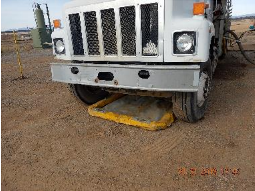
Photo 3: Containment under pump truck.
