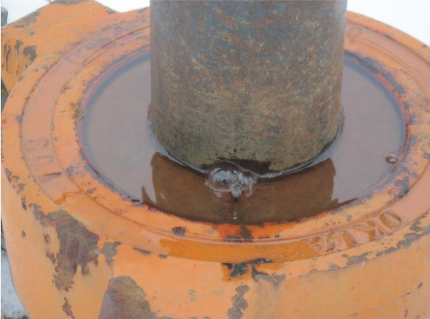
**Wellhead cap leaking**
