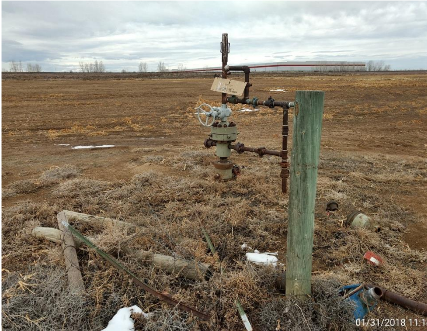
Wellhead Corrective Action: Unused equipment at wellhead, comply with 603.f
