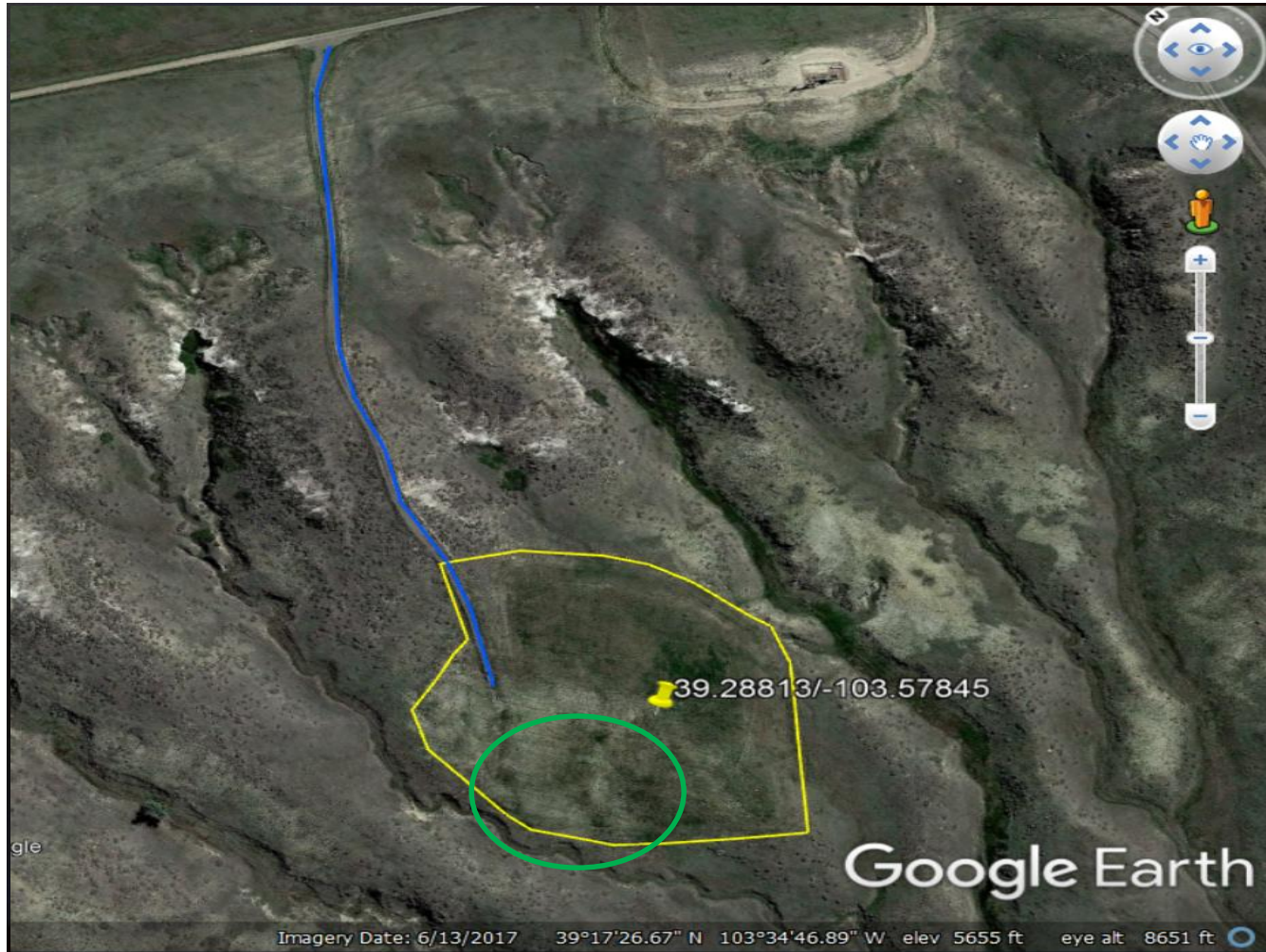
Photo 17: Aerial imagery (2017). Photo shows the location (yellow), areas of access road requiring reclamation (blue) and areas where erosion degradation is occurring (green).
