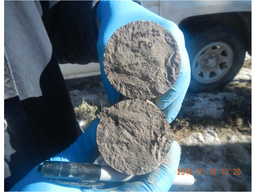
Core from 170 feet bgs. No odor or staining identified during drilling and coring of this well.
