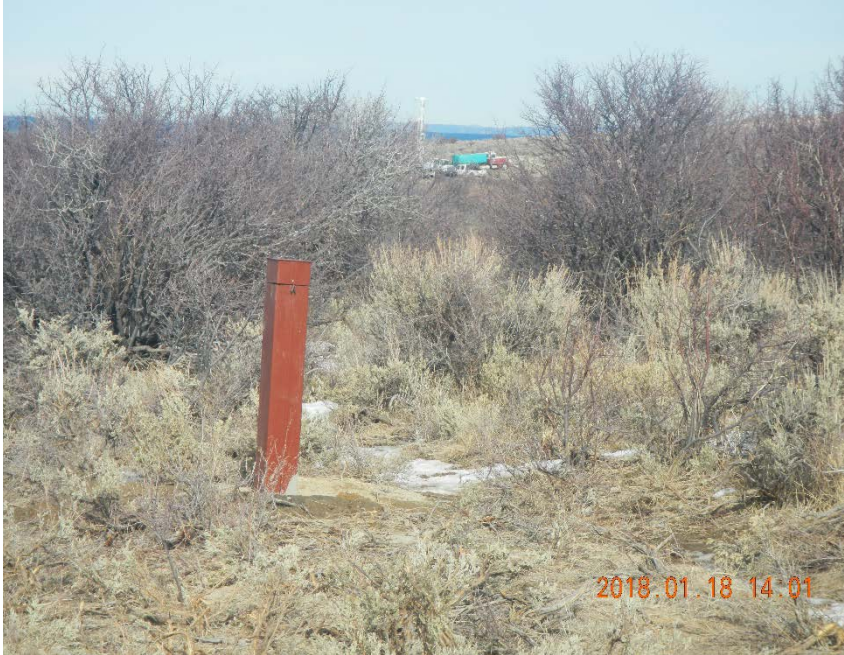
MW-20. Located approximately 900 ft north-northwest of the release point (on Divide Rd.) Free-product has been detected in this well.
