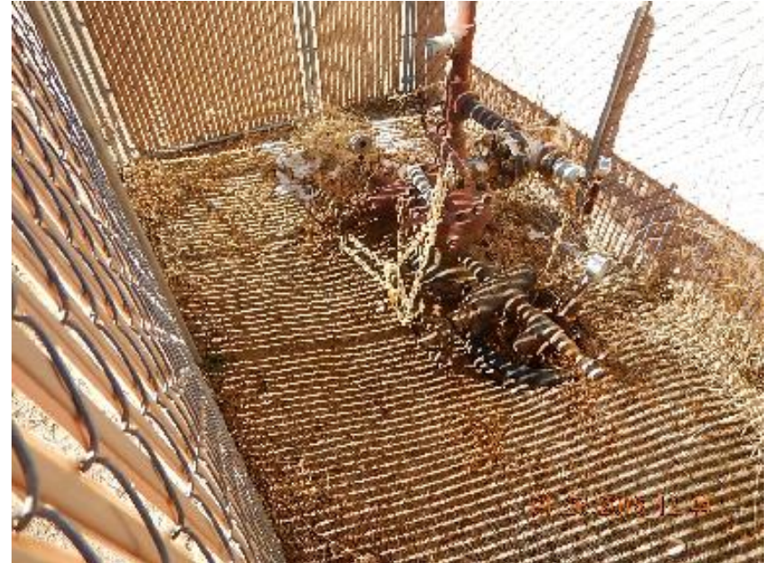
Photo 4: Fenced in wellhead with valves chained.
