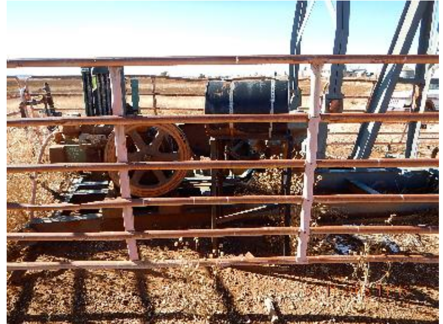
Photo 10: Lube oil tank with no spill prevention.
