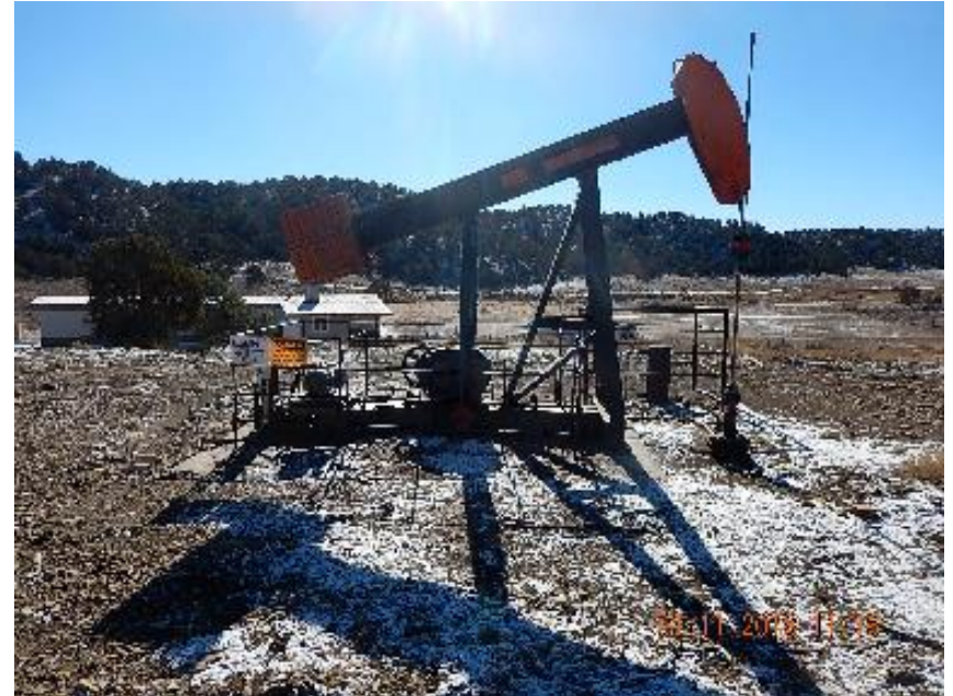
Photo 2: Pump jack, wellhead, and electric motor.
