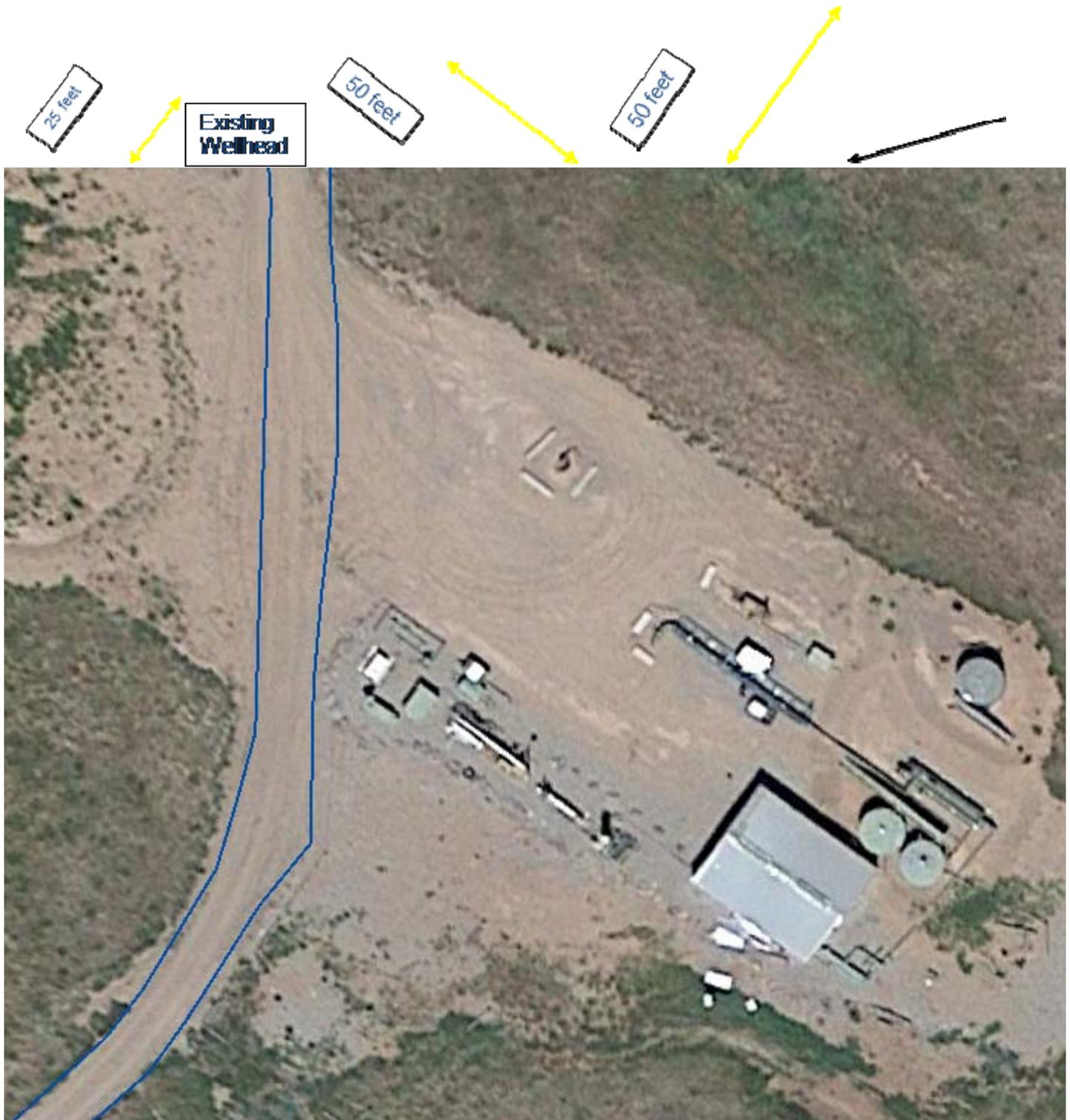
As can be seen from this view, the existing producing well is only 25-50 feet from the gas metering equipment and the edge of the reclaimed location. There's barely enough room to drive a truck around the wellhead; the existing pad area is about 75 feet by 100 feet, with the well near the middle, with no room for a drilling rig.
