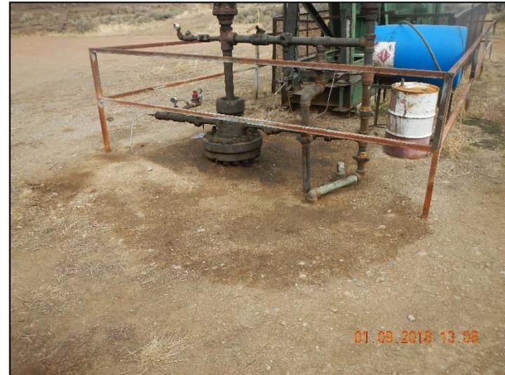
**Photo 2. Stained soil at wellhead and chemicals without secondary containment.**
