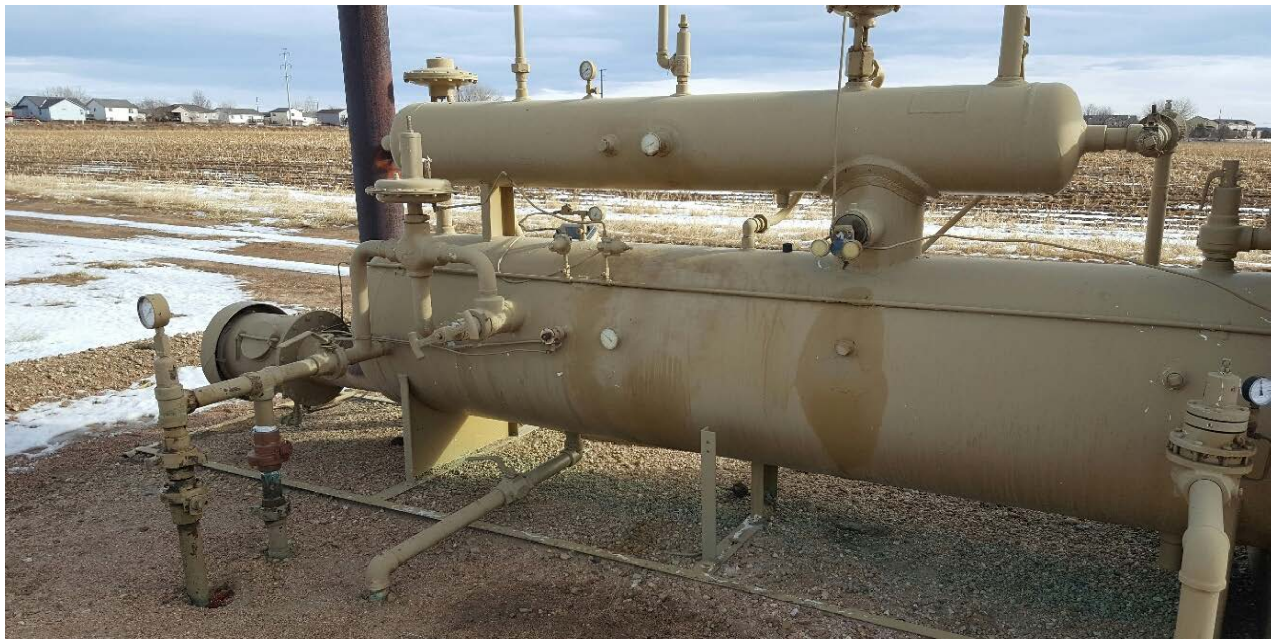
Figure #2 Fixed and cleaned leaking fittings
