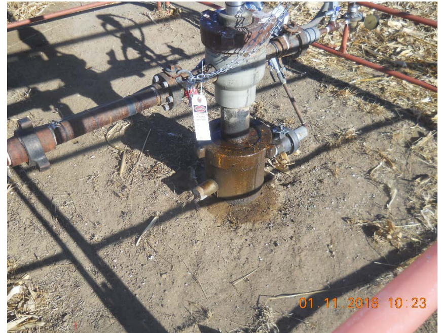
Stained soil around wellhead needs cleaned up
