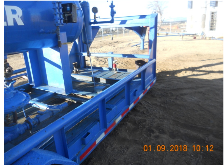
Photo 8. Knockout trailer cleaned. Fire extinguisher no tags
