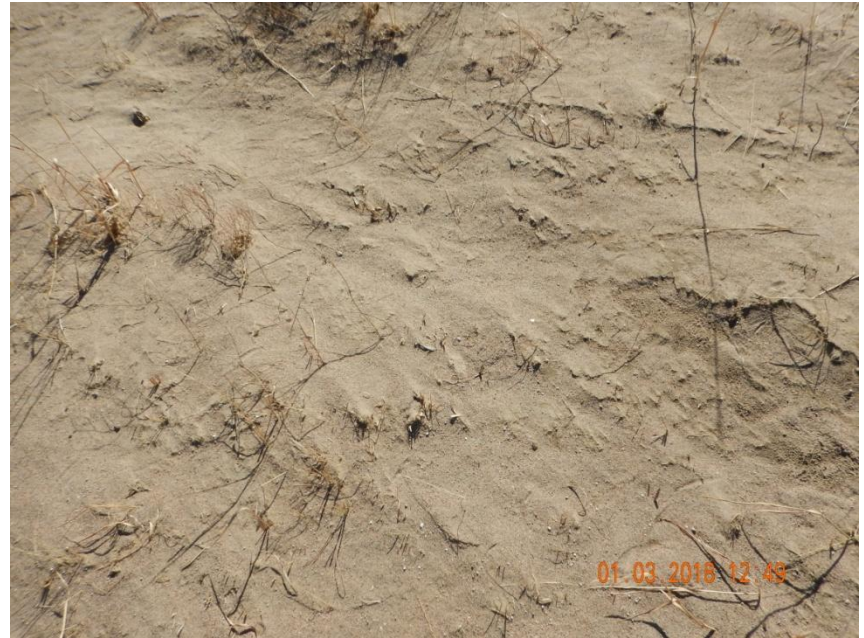
Photo 19. Close-up photo taken east of the location illustrating the evidence of sediment discharge off location.
