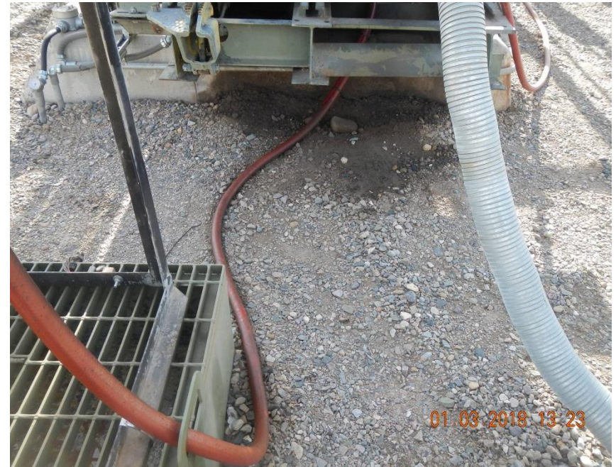
Stained soil beneath prime mover for #2 pump jack.
