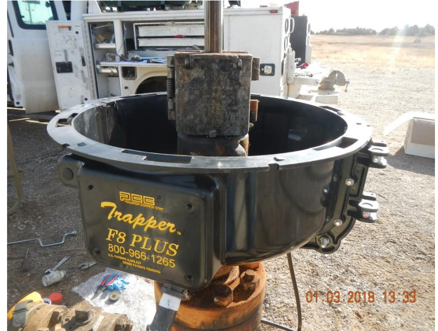
Float controlled trap being installed on well #4.
