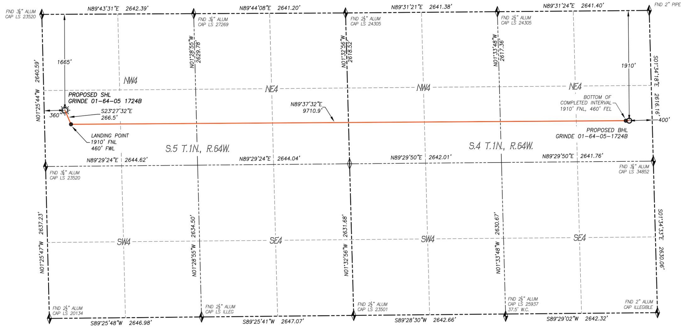
IN ACCORDANCE WITH A REQUEST FROM BILL BARRETT CORP., DALEY LAND SURVEYING, INC. HAS DETERMINED THE SURFACE LOCATION OF THE GRINDE 01-64-05-1724B WELL TO BE 1665' FNL, 360' FWL, AS MEASURED AT NINETY (90) DEGREES FROM THE SECTION LINES OF SECTION 5, TOWNSHIP 1 NORTH, RANGE 64 WEST AND THE BOTTOM HOLE LOCATION TO BE 1910' FNL, 400' FEL, AS MEASURED AT NINETY (90) DEGREES FROM THE SECTION LINES OF SECTION 4, TOWNSHIP 1 NORTH, RANGE 64 WEST, OF THE 6TH PRINCIPAL MERIDIAN, WELD COUNTY, COLORADO.
