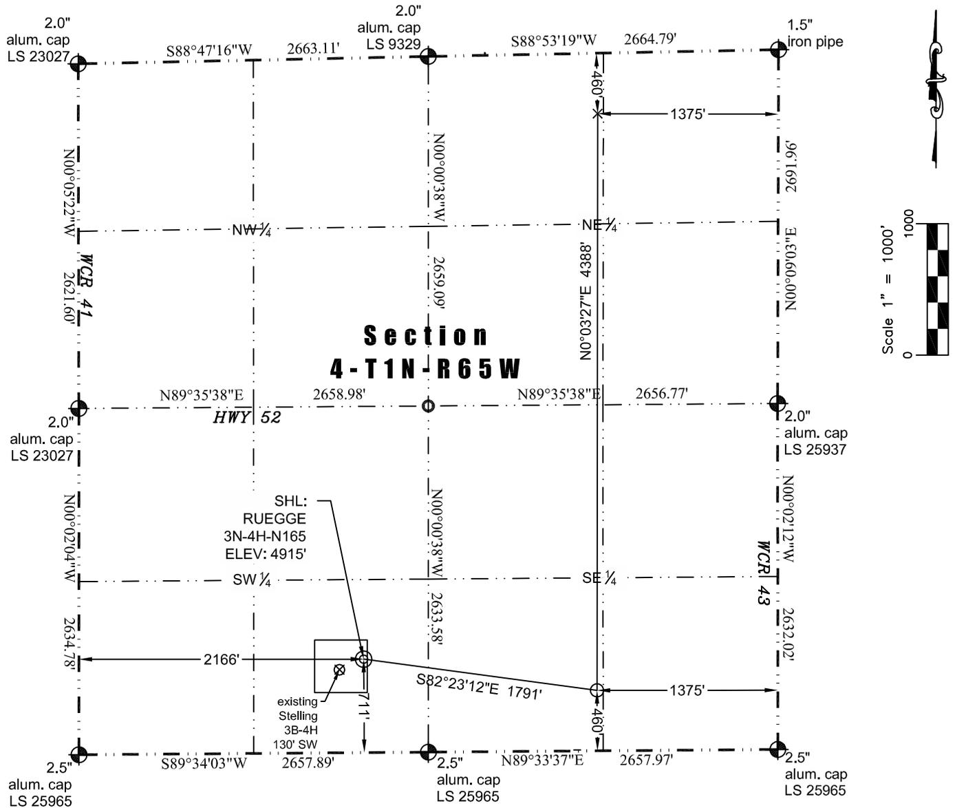
In accordance with a request from Jay Knutson of Crestone Peak Resources, Washburn Land Surveying, LLC has determined the location of the **RUEGGE 3N-4H-N165** well site to be SHL: 711' FSL and 2166' FWL, (TPZ: 460' FSL and 1375' FEL), (BHL: 460' FNL and 1375' FEL), as measured at ninety (90) degrees from the section lines of Section 4, Township 1 North, Range 65 West of the 6th Principal Meridian, Weld County Colorado.
