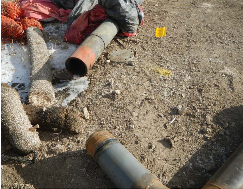
Failed Frac line elbow
