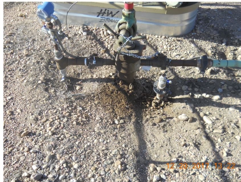
Stained soil under master valve needs cleaned up
