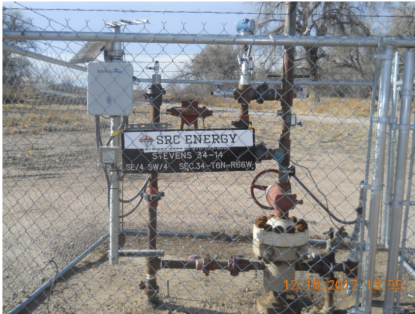
Wellhead looking west, no emergency contact information
