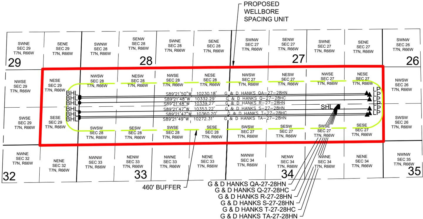
**G & D HANKS QA-27-28HN WELL TO BE LOCATED 1273' FSL AND 1574' FEL, SEC 27, T7N, R66W**
