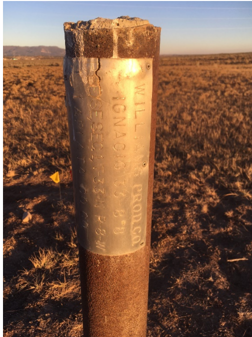
Photo 1. Plugged and abandoned well marker.
