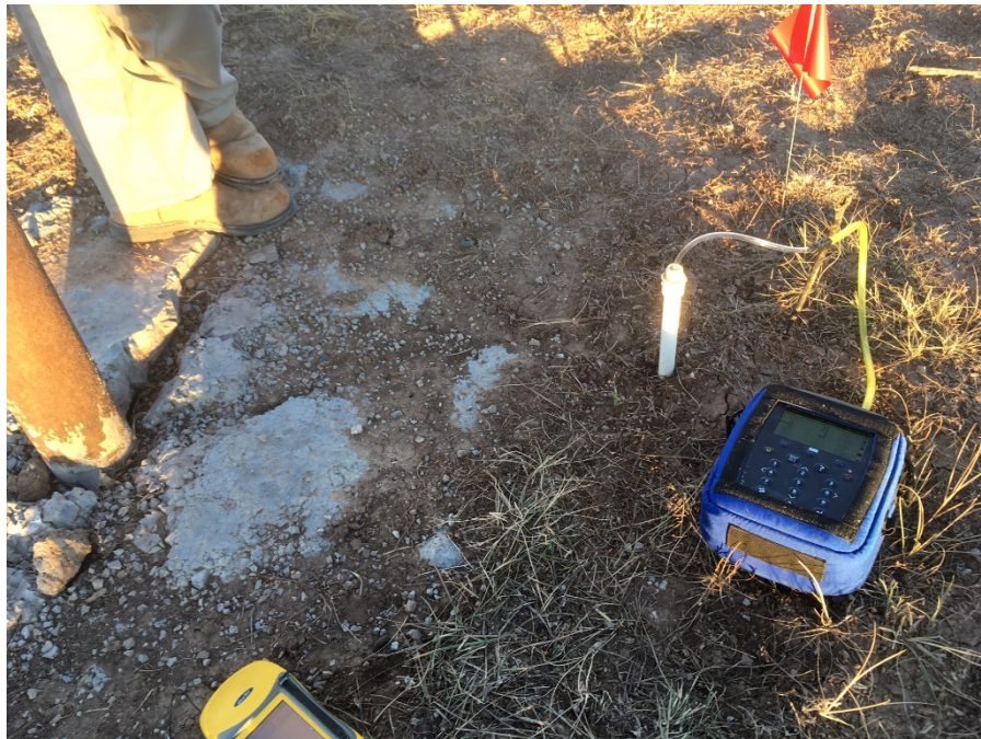
Photo 2. Soil gas measurement instrumentation and soil vapor tube next to abandoned well marker.
