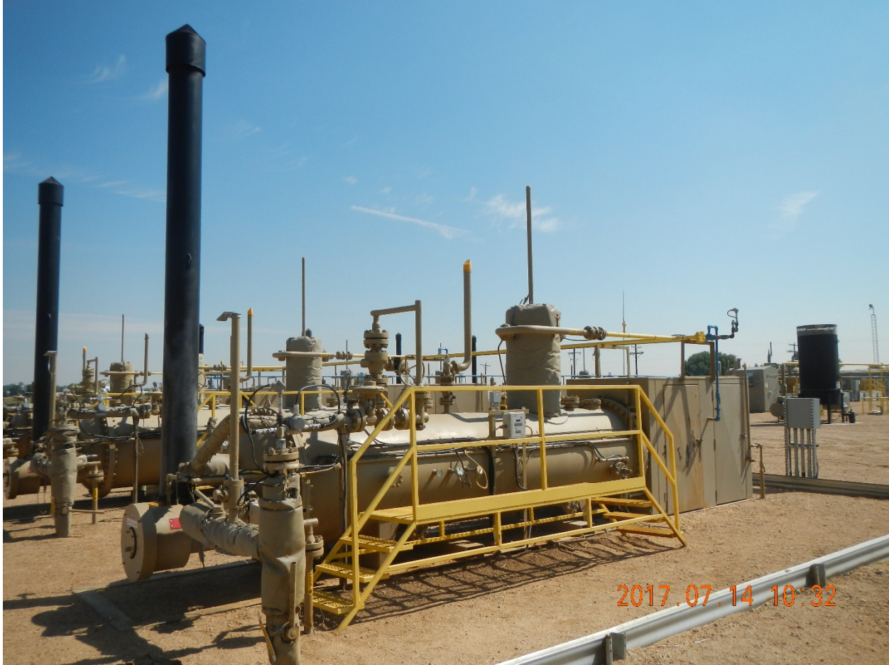
Horizontal Separator, a pop off valve on which was the release point for the plume observed by the complainant.
