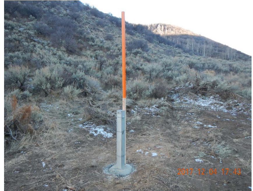
One of the monitoring wells installed by Caerus. Orange sticks differentiate Caerus wells from Encana wells (have yellow sticks).
