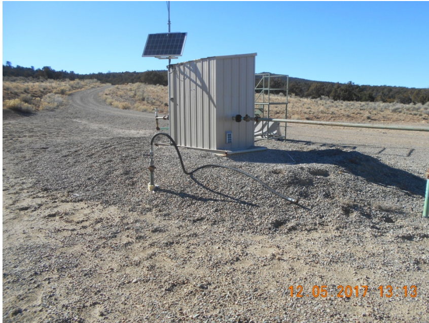
Unused riser with hose attached.
