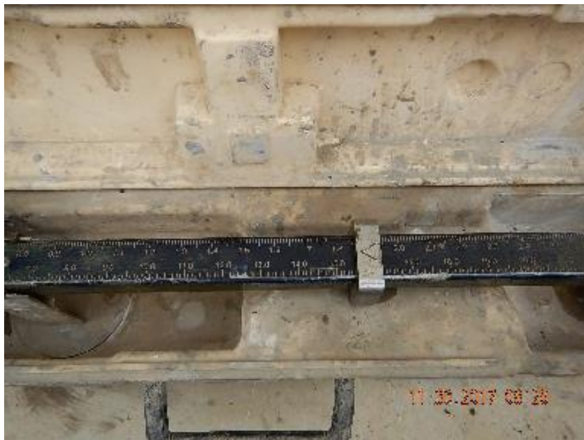
Photo 3. Mud weight verification check.
