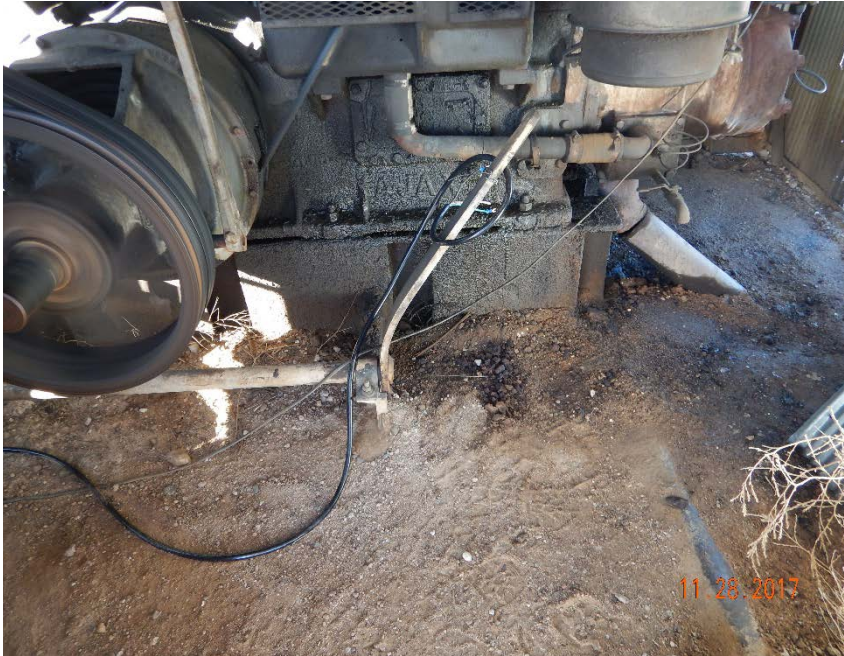
Photo #5 – Historical accumulation of oil-stained soil beneath prime mover.
