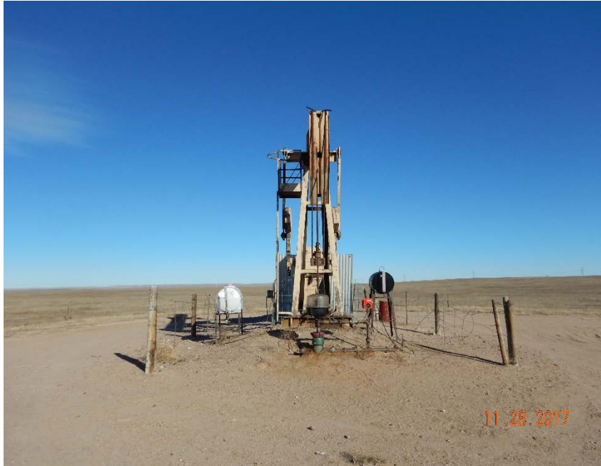
Photo #1 – View of wellhead and pump jack from south. Note localized accumulation of oily waste beneath wellhead and lack of secondary containment devices beneath day tanks.
