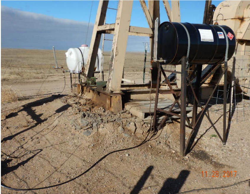
Photo #3 – Historical accumulations of oil-stained soil beneath day tanks at south end of pump jack. Day tanks lack secondary containment devices.
