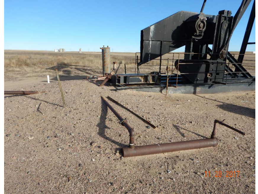
Photo #4 – Pump jack is not in use and lacks a motor.
