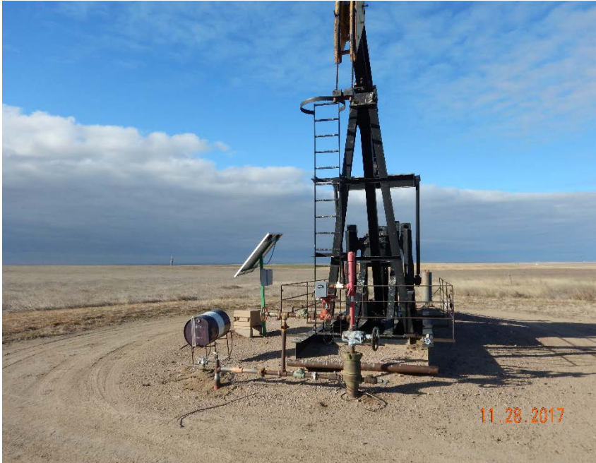
Photo #1 – View of wellhead and pump jack, looking west. Note that the well is equipped with a plunger lift and that the day tank south of the well is lacking secondary containment. There is no well sign at the pump jack.
