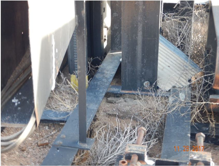
Photo #5 – Accumulation of wind-blown weeds and debris remaining beneath pump jack.
